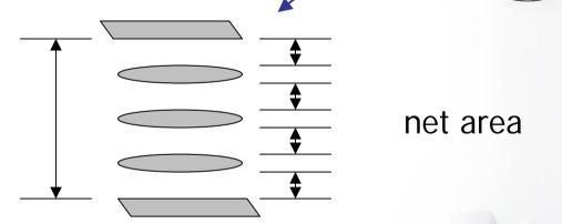
In the cp-value component the gross area should be used, since pressure drops which are due to the shape of the grille are modeled in the area resistance describing the grille.
