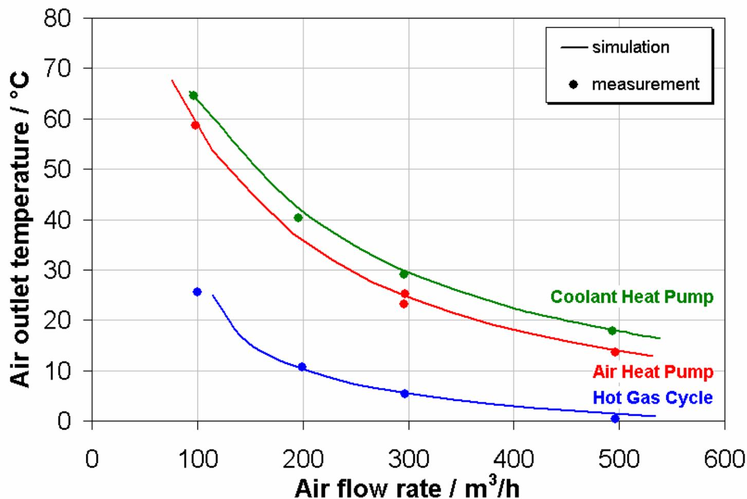
$t_{amb} = -5 \text{ }^{\circ}\text{C}$ ,  $n_{Com} = 900 \text{ rpm}$
