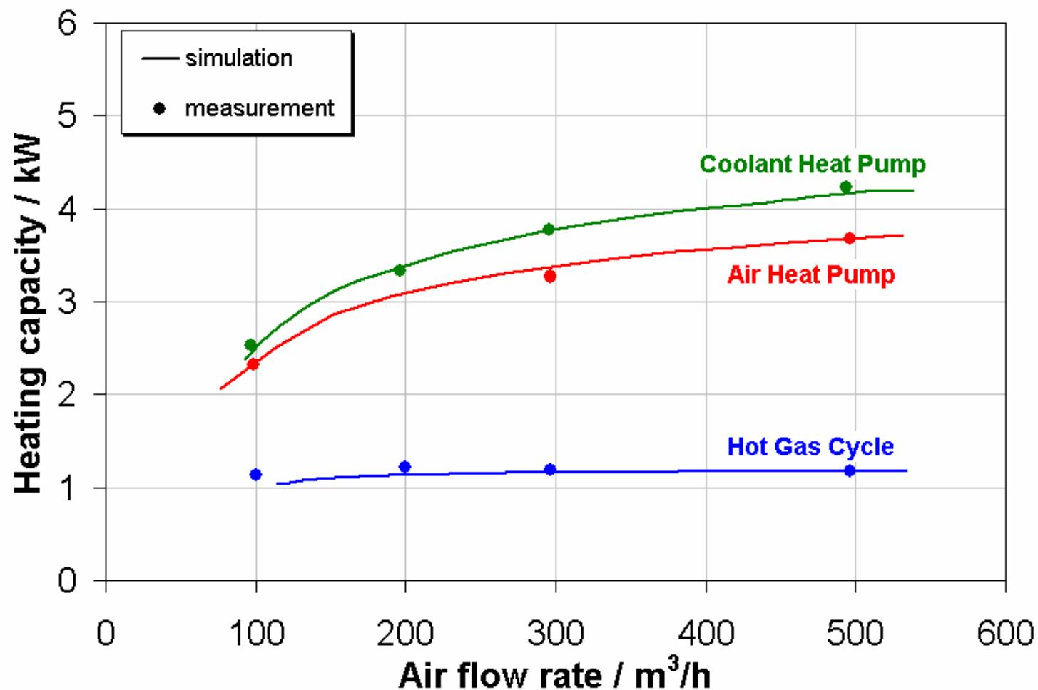
$t_{amb} = -5^{\circ}\text{C}$ ,  $n_{Com} = 900 \text{ rpm}$
