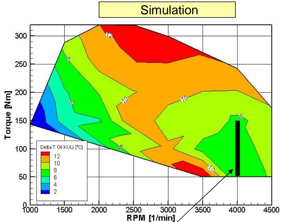
Section, where engine model was calibrated
